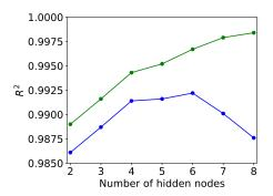
Figure 4: Determining the optimal number of hidden nodes for the boiling point. Green curve represents training  $\mathbb{R}^2$ , while the blue curve represents the cross-validation  $\mathbb{R}^2$ .
