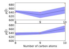
Figure 15: Cross-validation of density at  $100^{\circ}$ C for 4-methylheptane, 2,6-dimethylheptane and 4,5-dimethyloctane. In the top figure, we show results obtained from the neural network architecture that uses only the molecular basis as input features. In the bottom figure, we show results obtained from the neural network architecture that uses molecular basis and density data at  $20^{\circ}$ C as input features.
