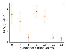
Figure 9: Average absolute deviation of the neural network model for the boiling point as a function of number of carbon atoms.
