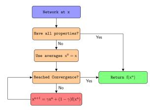
Figure 3: Data imputation algorithm for the vector x. We set  $x^0=x$ , replacing all missing entries by averages across each assay and, then, iteratively compute  $x^{n+1}$  as a function of  $x^n$  and  $f(x^n)$  until we reach convergence.
