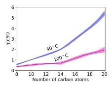
Figure 16: Blue/cyan plot shows predictions for the kinematic viscosity at 40°C while black/magenta shows predictions at 100°C.
