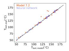
Figure 5: Parity plot for boiling point of alkanes. Our neural network model is compared to the model 7.2 from [33].
